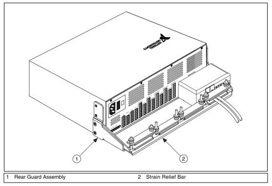
Figure 23. MID-7654/7652 with the Strain-Relief Bar Installed
